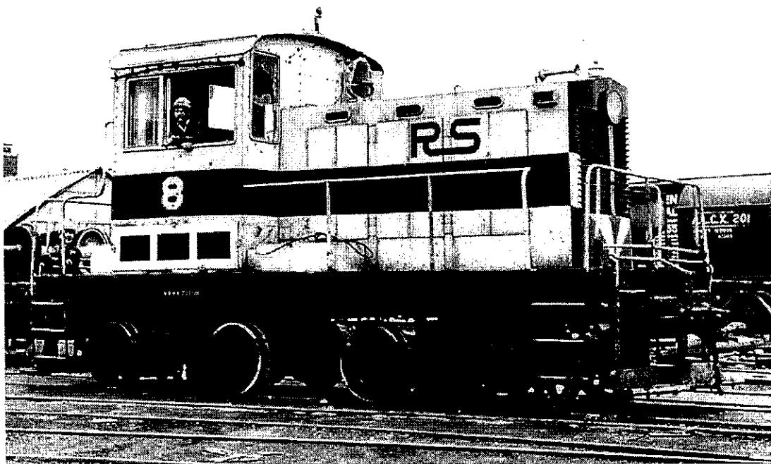
A much rebuilt shop switcher that was first an electric as number 6, then in 1941 a homemade rebuild diesel-electric with wheel arrangement of 1A-1A. It was rebuilt in 1950 as a battery-electric shop switcher.
