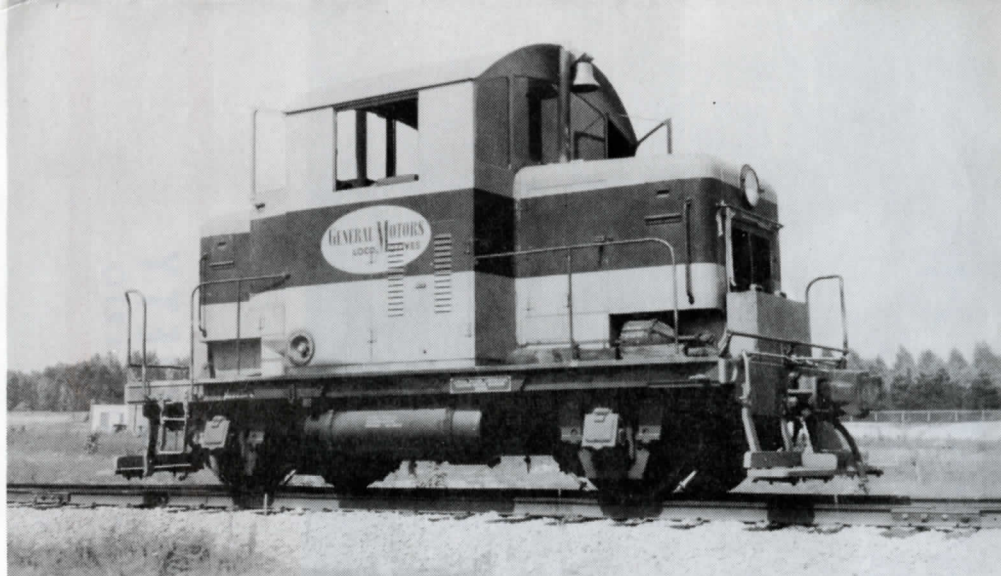
McKinnon Industries' unusual diesel-electric switcher is pictured at the Meritton, Ont. plant of McKinnon, July 16, 1951. The diminutive locomotive, completed by EMD on Aug. 2, 1940, serial no. 1134, is a Model 40. It was acquired from EMD's La Grange, Illinois plant in Feb., 1951. The unit has two traction motors and two diesel engines. --Ray Corley photo
