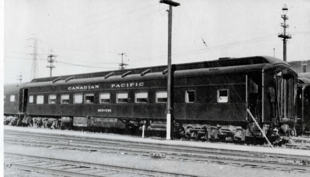
CPR sleeper "Redvers", pictured at John St. Coach Yd., Toronto, circa 1970, is similar to the sleeping cars recently acquired by the B.C. Transportation Museum (see Short Items). The eight section, two compartment, one drawing room sleeper was one of 29 such cars built by National Steel Car/CPR Angus Shops in 1929. --John D. Thompson photo
