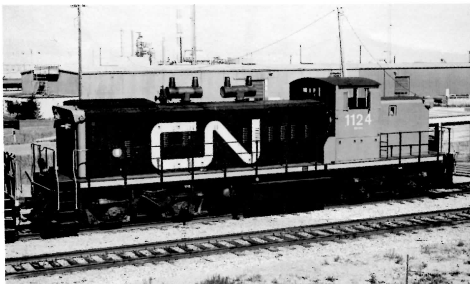
CN GMD-1 1124 has now been rebuilt to a B-B wheel arrangement and renumbered from 1024. Because the units are now on Flex-coil trucks and the GMD-1s had their sand boxes on the old trucks, the shops had had to construct body-attached sand bins and loading pipes to the rebuilt units. With the upgrading of many Western lines the need for C-C wheel arrangement units has declined. Clover Bar (East Edmonton), June 13, 1986.
