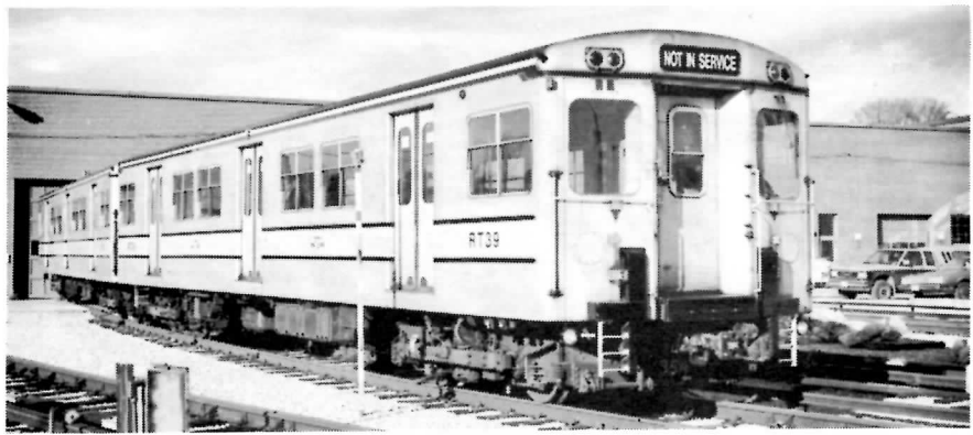
TTC Refuse Collection Cars RT38-39 pose at Greenwood Shop on Nov. 6, 1987, the day they officially entered service. They were formerly Gloucester Railway Carriage & Wagon Co. aluminum subway cars 5100-5101. The cars feature a wide yellow band (TTC work equipment colour) beneath the windows.
