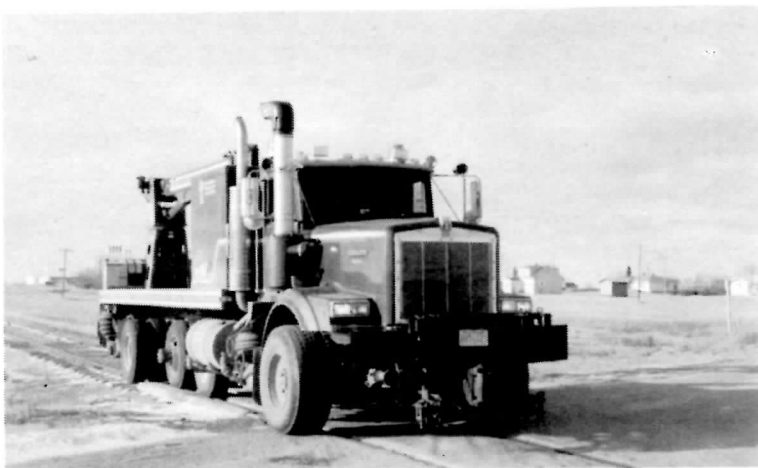
▲ The Brandt Road-Railer at Parry, Saskatchewan ▼ Engineer Norm Howse retracts the railway wheels
