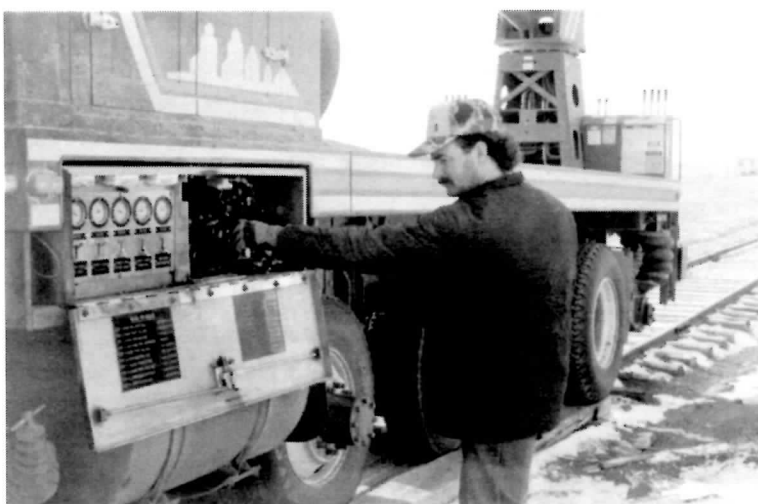
▲ The Brandt Road-Railer at Parry, Saskatchewan ▼ Engineer Norm Howse retracts the railway wheels
