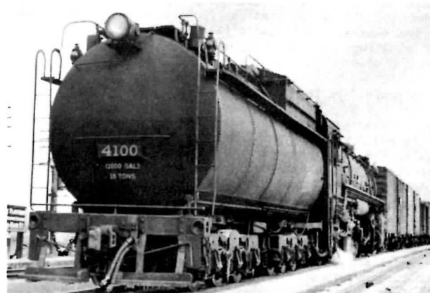
It takes a big tender to feed a big engine, and the 4100's can take sixteen tons of coal and eleven thousand gallons.
