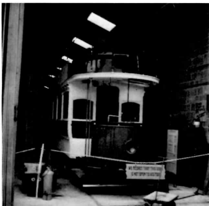
Parked inside the works shed is Southampton #45. This tram was the first tram at Crich, and is now undergoing an extensive overhaul before it will be resored to service. (L. Partridge)
