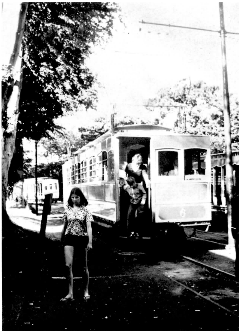
ABOVE: Snafell Mountain Railway #6 at Laxey where the SMR and MER meet. The SMR cars use bow collectors in contrast to the poles on the MER. The SMR cars and the enclosed cars of the MER have the unusual door placement. BELOW LEFT: IOMR Station at Douglas. This impressive building is the main station as well as the railway offices. Unfortunately, the signs on the posts read "Service to Port Erin from Castletown-No Trains from Douglas this year." BELOW RIGHT: Joint SMR-MER station at Laxey. All Sept 75 (DWS)
