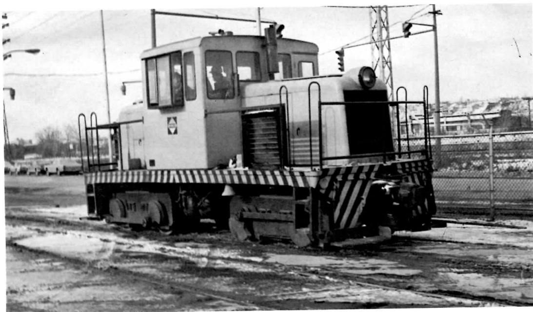
This GE 45-tonner belongs to Sidbec-Dosco and operates at its Montreal plant. (P. Patenaude)
