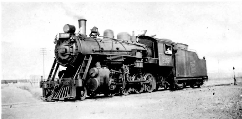
ABOVE - Mikado #3564 was a member of class S-2-b from leaving CLC in 1923 to scrapping late in 1961. Starting out life as coal burners, they were converted to oil in 1953-54. 3564 is shown here in Winnipeg in July 1947. (UCRS coll.)
