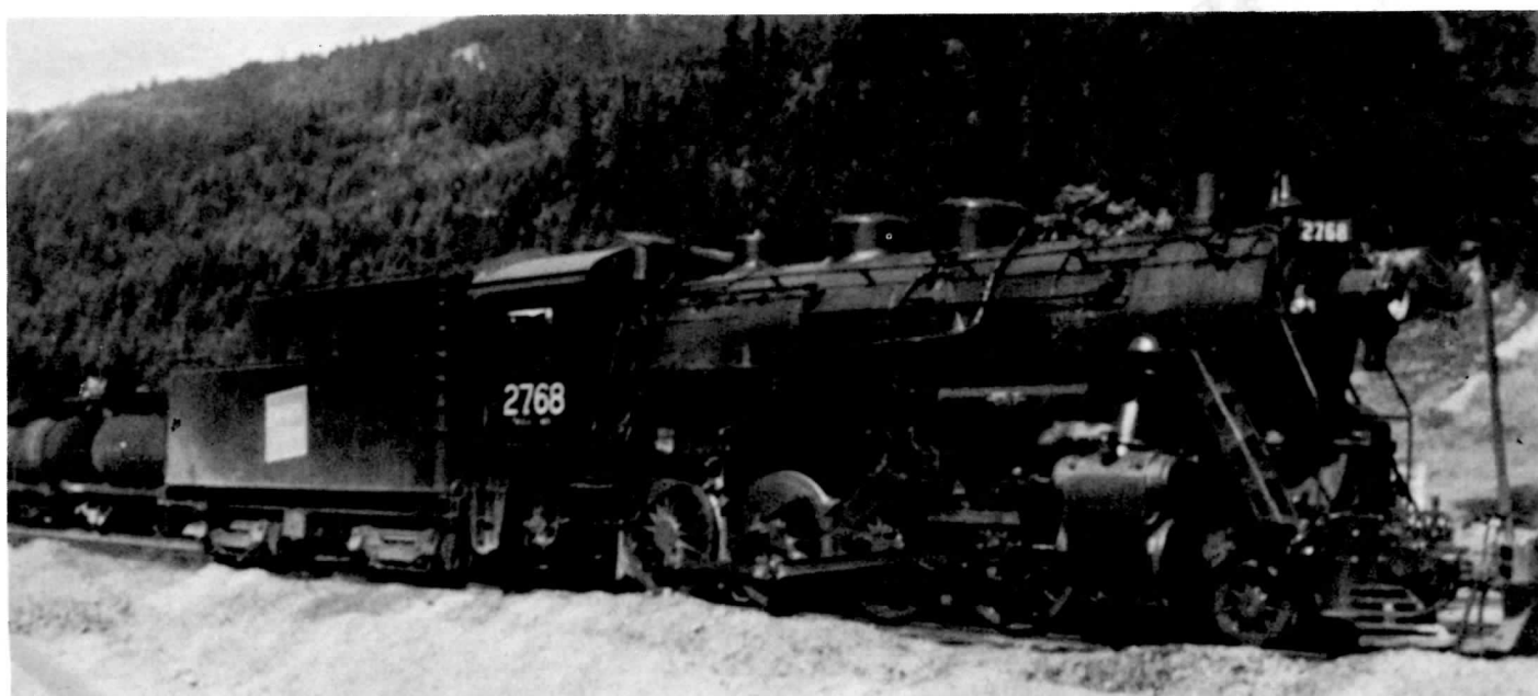
BELOW - With the mountains for company CNR 2-8-0 #2768 is seen here in a siding in B.C. Part of class N-5-d, the locomotive was built by CN at the Pointe St. Charles shops in Montreal being outshopped in October 1931. 2768 was the first of her class to be scrapped in July 1954. (UCRS coll.)
