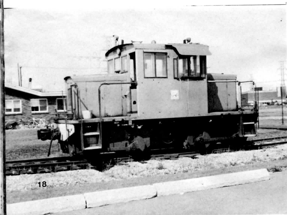
Atlas steel's GE 43-tonner is currently the oldest operating GE unit in Canada. Built in 1939 it was formerly Wabash #51 and was stationed at St. Thomas, Ontario. Pictured here at Tracy, Quebec. (P. Patenaude)
