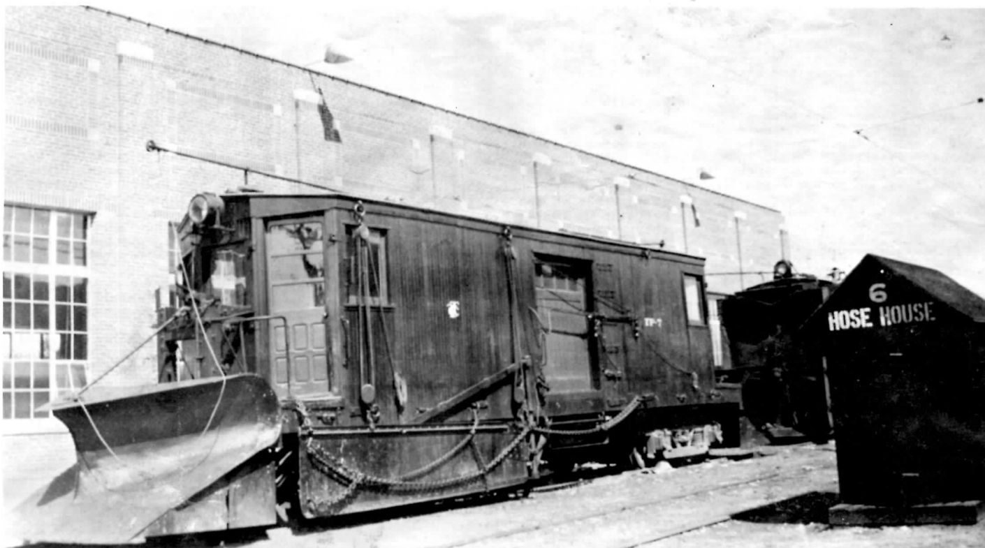
The TTC's little used North Yonge plow TP-7, formerly Toronto & York Radial Rly. #7. Seen here at Eglinton carhouse in 1938. The car was scrapped in 1946 and its trucks were placed under the front of crane cars C1 and C2. (J. Knowles)
