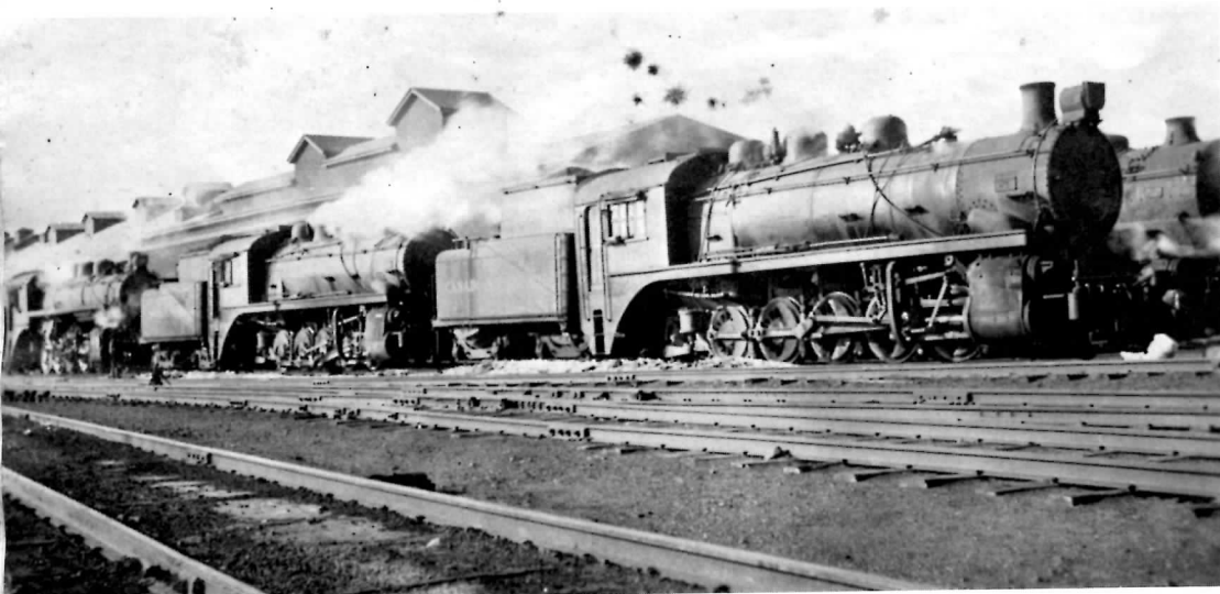
Class W1a were the only 0-10-0's in service on the CPR. Built by CP at Angus in 1914, the entire class is shown here at Winnipeg on May 15th. 1940. Closest to the camera is #6950. (UCRS coll.)
