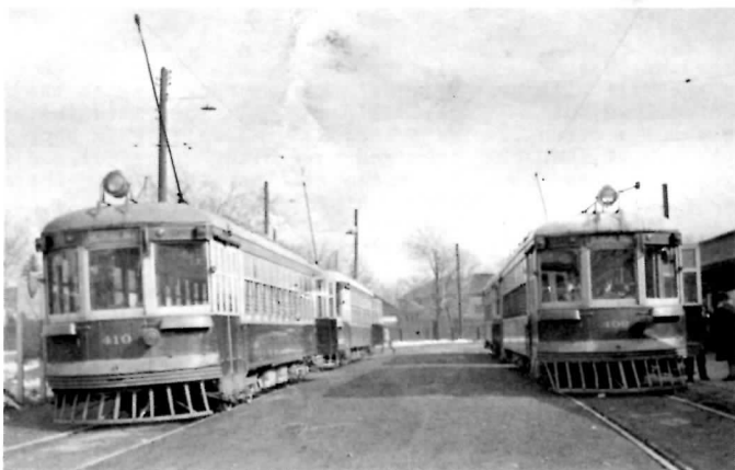
BELOW - Car #412 loads at Glen Echo in 1939. The shedman sent up from Eglinton Division walks on the roof installing sleet cutting wheels to the trolley poles. (J.D. Knowles)
