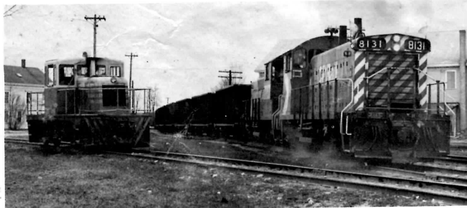
BELOW CP Rail SW-1200RS #8131 in DAR service at Hantsport, N.S. on the head end of the gypsum train. On the left is the Canadian Gypsum Company's GE 45 ton switcher which handles the cars (six at a time) on company tracks. (K.A. Gansel)
