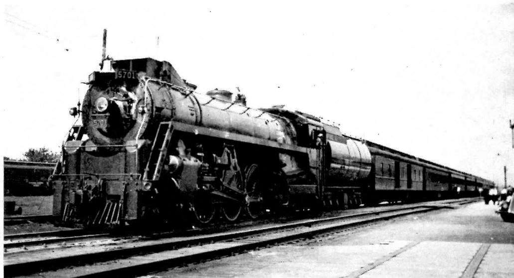
Mainstay of the Toronto - Montreal passenger services in the '30's and '40's were the CNR K-4-a Hudsons. With extra large water tanks to make the 100 mile Toronto - Belleville - Brockville - Montreal hops, they were built by MLW in 1930. Number 5701 is caught at Oshawa, Ontario heading up the west-bound #5. 5701 was scrapped in November 1961. (R. Hope)
