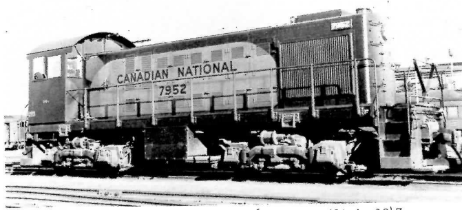
Alco S2 #7952, originally classed Q-6-a, was built in 1947. Reclassified MS10-a, it was retired in October 1973 as #8118. Shown here in the as delivered black and orange paint scheme.
