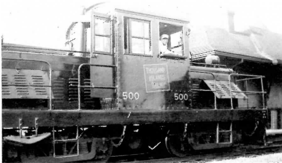
Thousand Islands Railway 500 was built by the Oshawa Railway shops with gasoline engines, replaced with diesels in 1948. It spent most of its life as TIR's sole piece of motive power. Retired in 1966 and now on display at Gananoque.
