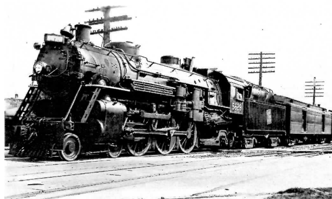
Grand Trunk Western 5629 was based on a USRA heavy Pacific design and was built by Alco in 1924. One of 5 K-4-a's it is now owned by Dick Jenson of Chicago.
