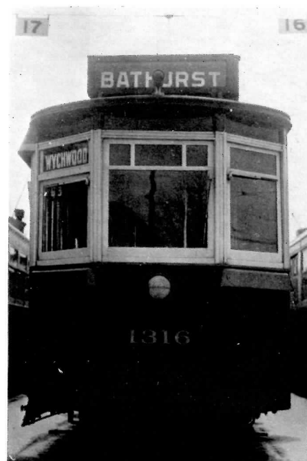
Toronto Transit Commission Wooden car 1316 at St. Clair Divisions Wychwood Carhouse. Originally built in 1910 by the Toronto Railway Company as an O-1 class car, it became TTC class BB in the 1932 reclassification. They were all withdrawn from service by the early fifties.
