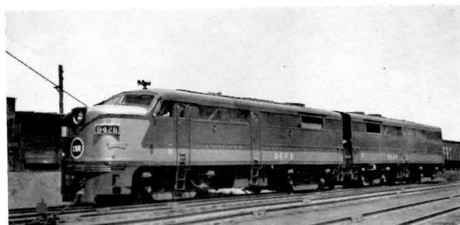
CN 9426-27, FA2 FB2 set was built by MLW in 1952. Used in freight service they were retired in April 1967 and May 1966 respectively. Shown in original paint scheme.
