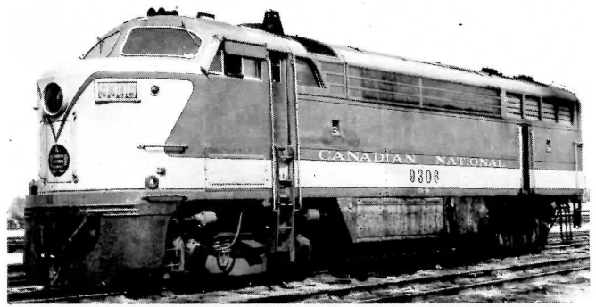
CN 9306 a CFA16-4 was part of the 20 unit order built by CLC in 1952. The unit was retired in January 1967. (D.W.Smith Coll.)
