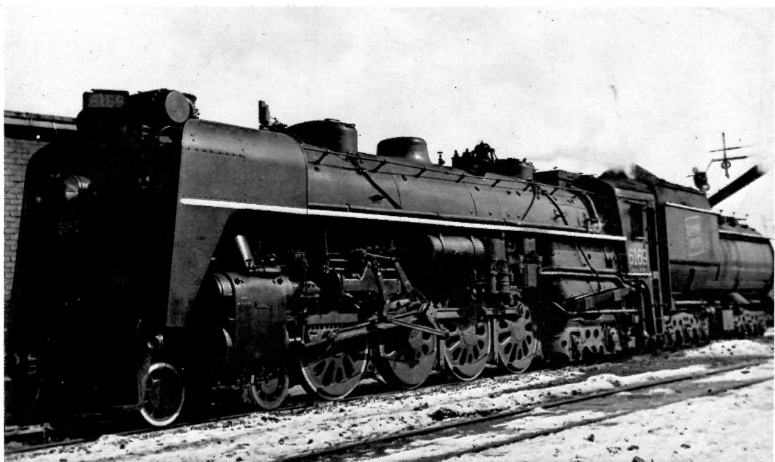
Taking on water is U-2-e Northern 6169. Built for CN by Montreal Locomotive Works in 1940, she was scrapped in 1955.
