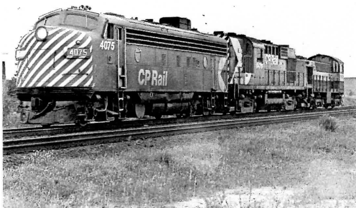
Canadian Pacific FP7A 4075 and RS 8479 trail behind the pilot engine taking them to Agincourt Yard. The units, off the Toronto section of the "Canadian", are maintained at Agincourt Yard and a pilot engine usually takes it there from John Street. Photo by Dave Booth at Birchmount Rd.
