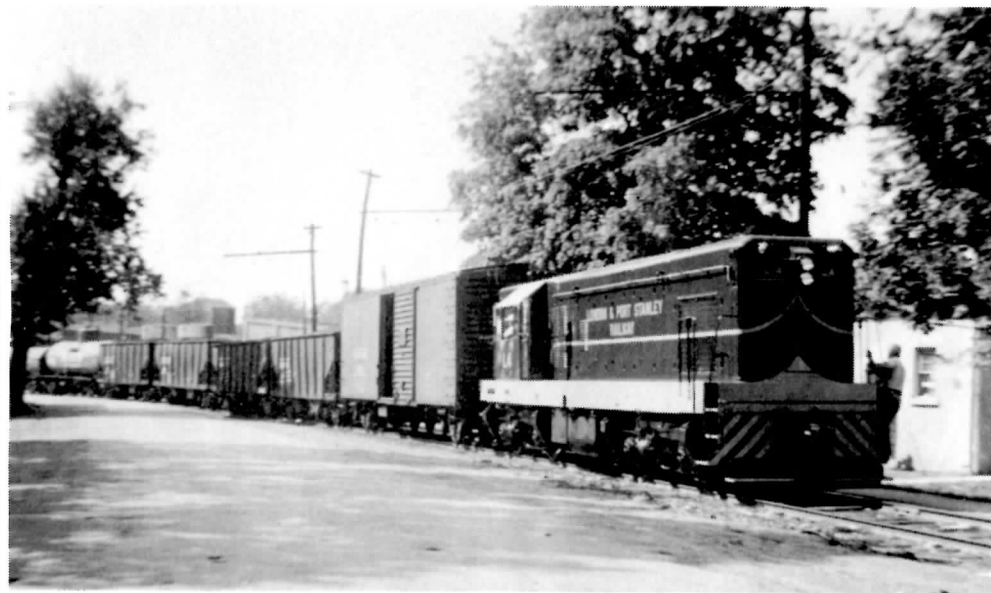
General Motors 1310 H.P. diesel locomotive L4 (later CNR 991), on its inaugural run on the L&PS, Sept. 15, 1955.
