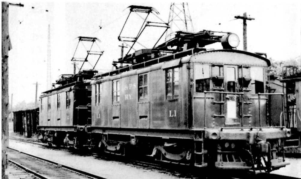
L&PS 60-ton box cab electric locomotives L1 and L2, CGE products of 1915, at the Phillip St. yard in London.
