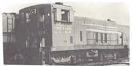
LEFT: No. 107, one of three G.E. 70ton diesel electrics on the S.F.P. & P. roster is shown switching at Kapuskasing. More modern steam engines were as follows:
