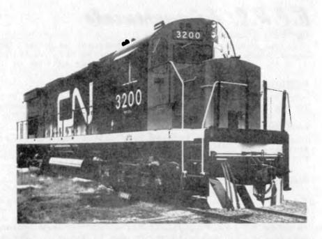
The newest diesel unit on the Canadian National, numbered 3200 and 3201, were first tested at Montreal Locomotive Works on November 17th, and made their first revenue run, to Toronto on Friday, December 4th. Following minor modifications at the manufacturer's, they made a second return trip to Toronto on December 10th. The units, C.N. class MRS-24a, are Century 424 series, 2400 h.p., B<sub>0</sub>-B<sub>0</sub> types.
