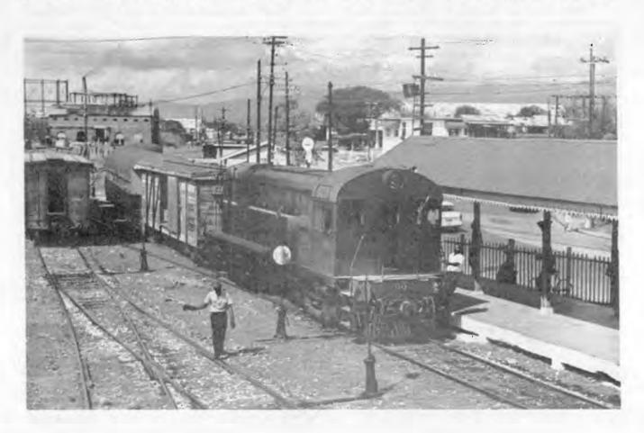
almost 800 ft. It is a winding climb which increases the effective gradient and when these factors are coupled with wet rail conditions it will be realized just how formidable was the task of the two 750 h.p. English Electric engines.
