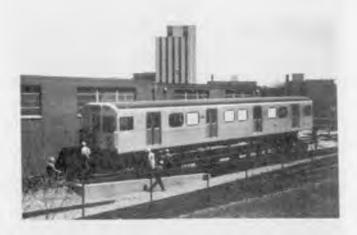
The unpainted exterior of the cars has a brushed aluminum finish. The roof is painted black and a black undercoating is used on exterior structure and components located below the carbody.
