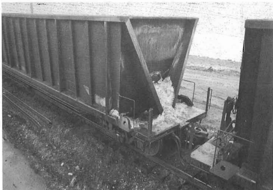
Solid bottom gondolas with swivel couplings, usually 105 gondolas to a train allow rotary dumping without uncoupling and permit continuous movement of the whole train.
