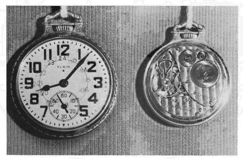
A more recent railroad watch design, Elgin No. 30,366,448 was made in 1927, but is still capable of passing railroad inspection. Note that the grade name "B.W. Raymond", introduced in 1867 and shown on No. 2042, is still used. The numerals 13 to 24 are on the inside of the watch crystal to adapt it for Canadian service. (C. De Jean).
