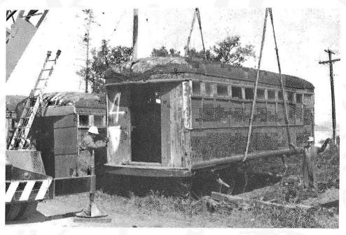
No. 134 is carefully lifted. Note the "rub-rail" at the bottom of the side to protect the car when in traffic. This car is in the best condition, and restoration will start with it. (Photo by R.D. Thomas).
