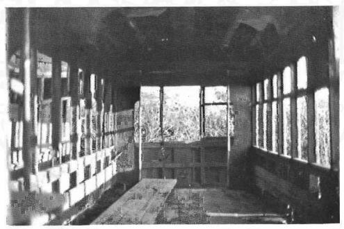
The interior of one of the 130-class cars just before being moved. The interior framing is visible and appears to be in good condition. (Photo by R.D. Thomas).
