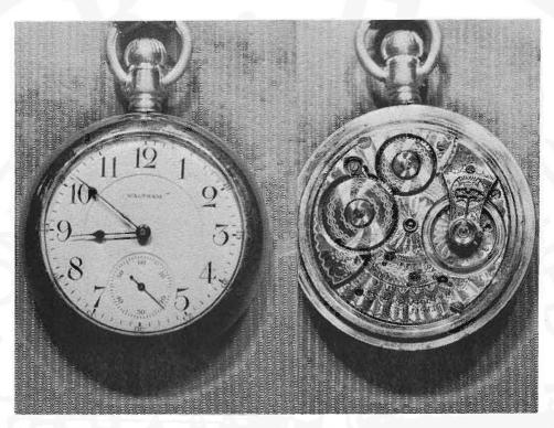
Waltham's answer to the new watch standards of the 1890's was the model 1892, designed from the start for railroad service. Shown here is No. 7,818,910 which was made in 1897. This watch is used by the author in regular service and can be depended on to keep time to within 30 seconds a month, even after 83 years service, a tribute to the workmanship of those days. (Photo by the author).
