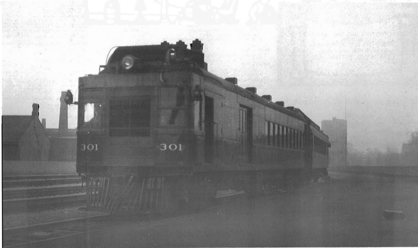
Like many North American railways during the 1920's, the TH&B bought a self-propelled car in order to reduce the cost of operating local passenger train service. Gas-electric car 301 spent most of its working life on the Welland-Hamilton-Waterford local train schedules. Pulling a wooden coach, 301 is shown departing Hamilton enroute to Welland. If all goes well, the arrival the train will arrive in Welland at 1710, one hour and ten minutes after the departure from Hamilton.
