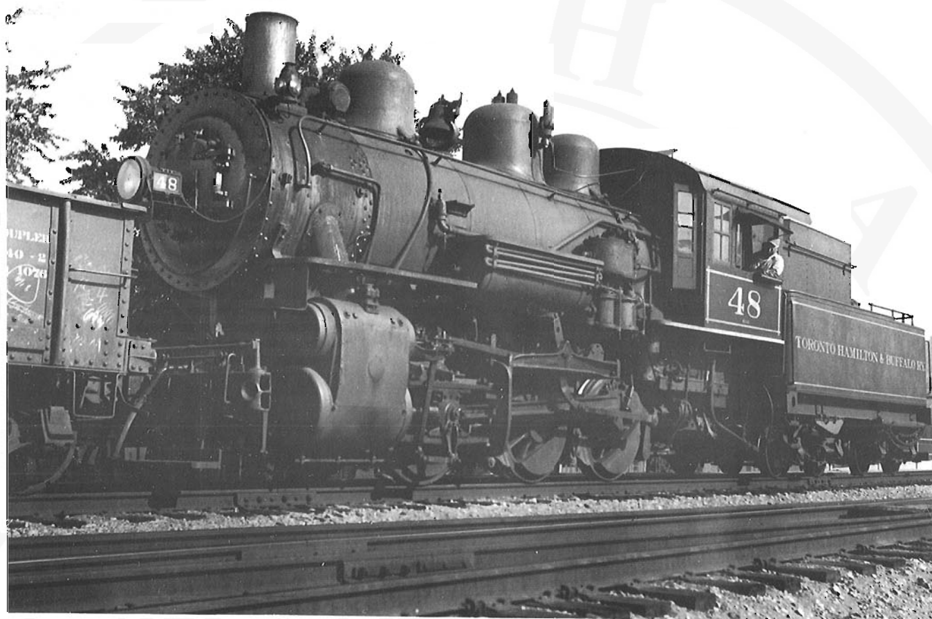
A large source for the TH&B freight revenues was the industrial district of Hamilton. In order to serve the many spurs and belt lines, the TH&B maintained twelve 0-6-0 switch engines. Locomotive 48 is shown showing a cut of freight cars in Hamilton on September 23, 1935. Number 48 was built by the Canadian Locomotive Company of Kingston, Ontario in 1917. Credit: Paterson-George Collection.
