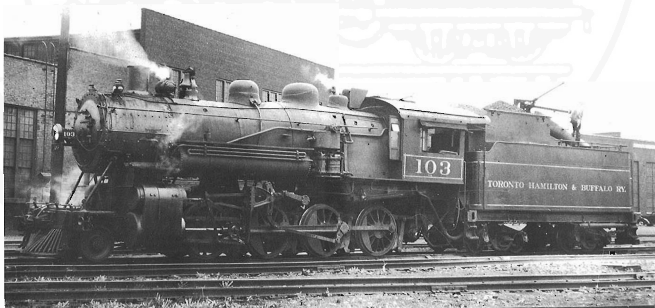
Consolidation 103 stands outside the Aberdeen roundhouse on July 22, 1948. The engine was built by the Montreal Locomotive Works in 1910 and originally bore the number 52. In January 1918, it was returned to MLW for installation of superheaters and emerged as Number 72. In 1919, it was renumbered 103. This locomotive is preserved in the Hamilton area.
