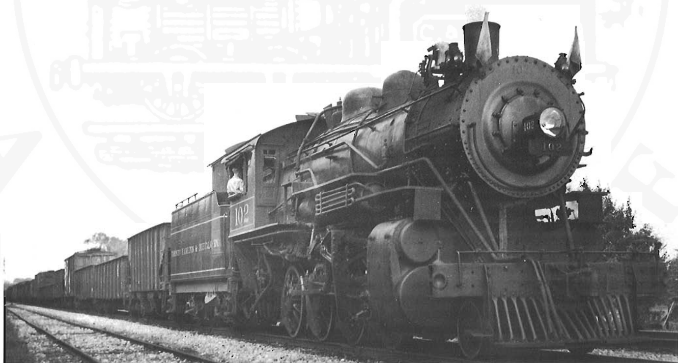
Prior to the arrival of the Berkshires, the biggest freight engines on the TH&B were 2-8-0 types. Locomotive 102 (original number 51) was built by the Montreal Locomotive Works in 1910 and could develop 45,780 pounds of tractive effort. This view taken on October 31, 1931 shows the engine on a freight train in Hamilton in a relatively unmodernized condition. Credit: Paterson-George Collection.
