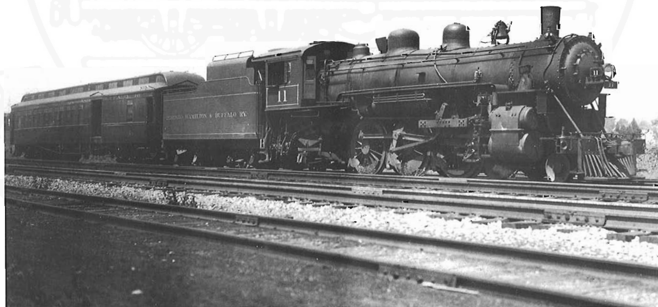
Some days the gas electric car was sidelined for mechanical reasons. On one such day in 1948, the local train from Hamilton to Waterford operated with a conventional consist. Shown at Waterford is Pacific 11 and a wooden combine which was retained for just this purpose. Locomotive 11 was built by the Montreal Locomotive Works in 1913.
