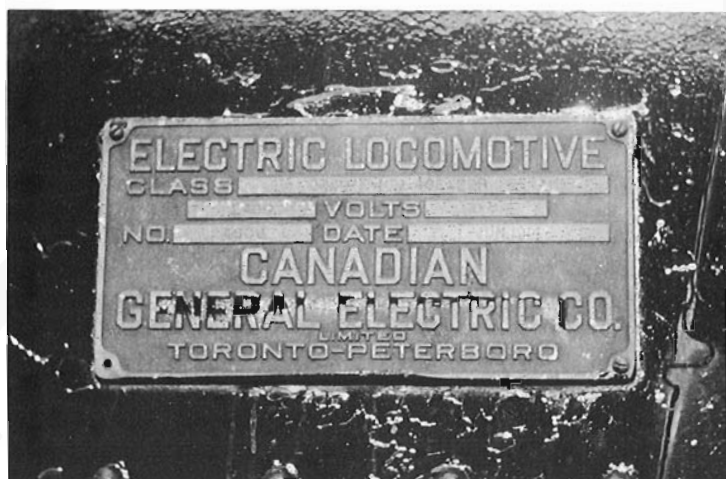
The builder's plate of 601 (then numbered 101) as seen, still on the locomotive, on October 20, 1968. The inscription reads: ELECTRIC LOCOMOTIVE Class 0440-E-166-4GE229B 2400 Volts D.C. No. 4609 Date Jun 1914.
