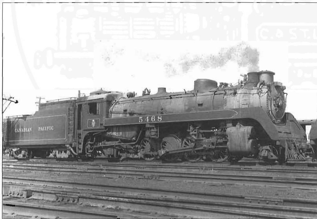
*The high pressure P2 class CPR 2-8-2 were high efficiency machines that could be found all across the system. Number 5468 was one of twelve Mikados built in late 1948 and was one of the last new steam locomotives built for the CPR. Through her brief career she called Kamloops, Revelstoke and Alyth Yard in Calgary her home terminals. Pictured here at Alyth circa 1956, 5468 is now the star exhibit from the CRHA collection at the Revelstoke Railway Museum. Dave Shaw Collection*
