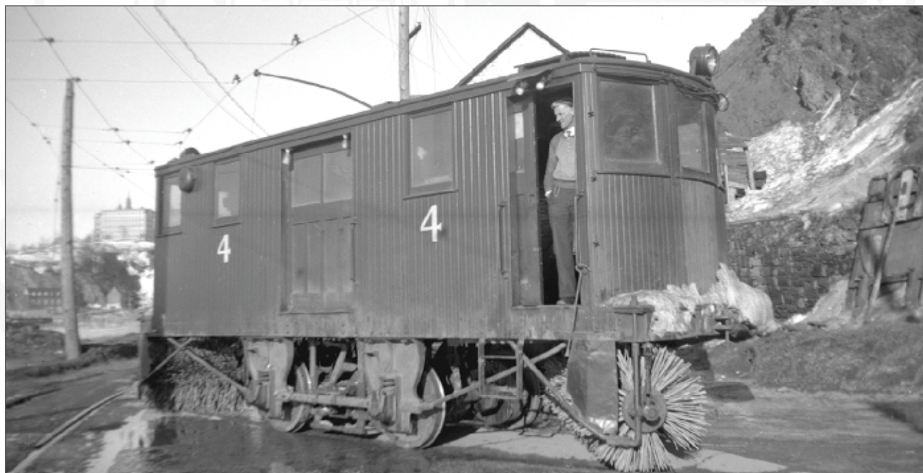
This double-truck sweeper (second #4 as first destroyed in 1921 fire) was acquired new in 1922 from the Russell Car & Snowplough Co. in Ridgeway, Penn. The sweeper is posing in front of the company's St. Laurent Street car barn in Lévis which opened in 1924. Al Paterson Collection
