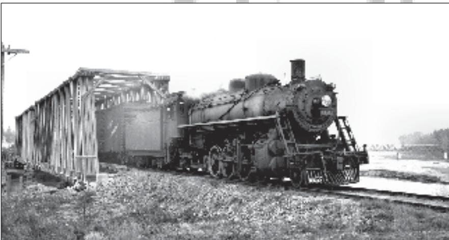
CLC 2-8-2 162 emerges from a wooden Warren truss bridge near Squamish, B.C. in 1950 with a CPR "Spans the World" 40 foot boxcar immediately in tow. No 162 was built in 1947 by Canadian Locomotive Company and was one the last new CLC steam locomotives built for a Canadian railway. By 1956, it was retired and scrapped. Ronald S. Ritchie.
