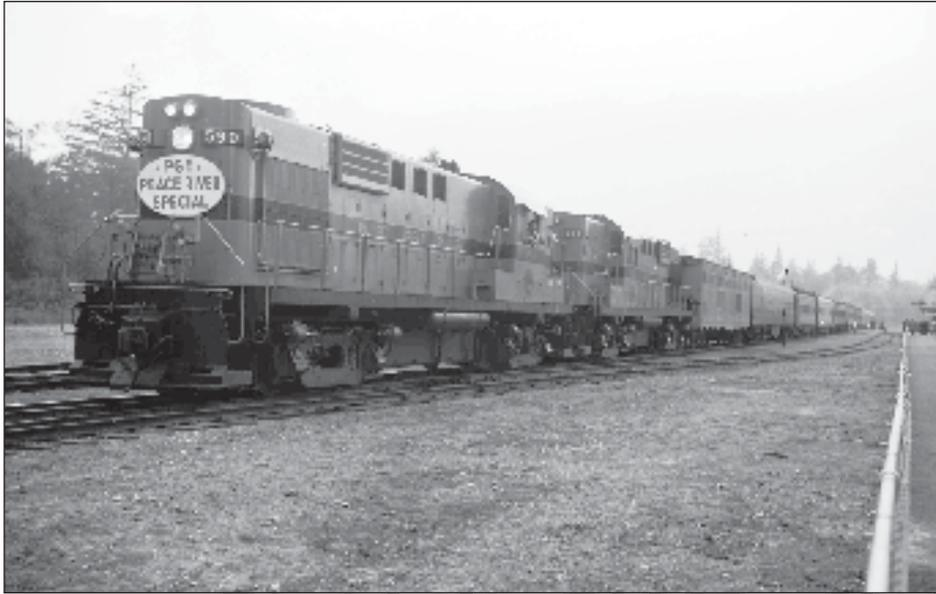
Number 590, an RS-11Mu, built by Montreal Locomotive Works in May 1958 is on the point of the Peace River Special, which officially dedicated the new line in October 1958. The 590 was renumbered to 604 and had a long life on the PGE; it was retired by CN in 2008. BC Archives collection, Call Number I-32406.
