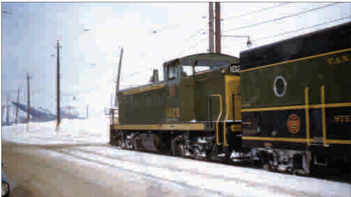
For a few years, after steam and before Rail Diesel Cars (RDC), the Murray Bay train service was handled by CNR GMD-1 class diesel locomotives. Here 1026 (a freight locomotive), is followed by an almost new steam generator car, which provided steam heat to the following coaches. Train 176 is standing at Ange Gardien under the QRL&P trolley wire en route to La Malbaie. Ronald S. Ritchie.
