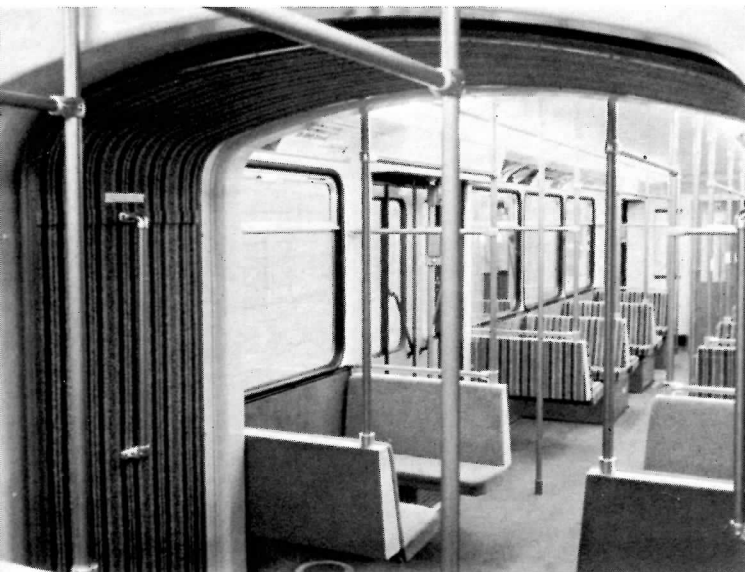
Both the walls and the ceiling area inside the articulated section are carpeted in the same orange/beige/brown combination as are the majority of the seats.
