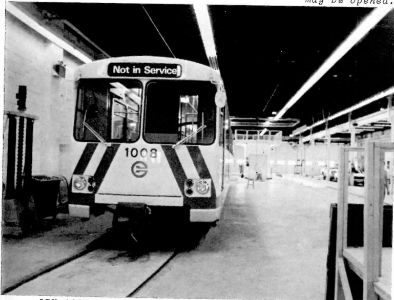
LRV 1008 poses inside Cromdale Shops. Dark stripes below the doors along the sides and diagonally across the front are a luminescent blue; below is a gold stripe, also running the entire length of the car.
