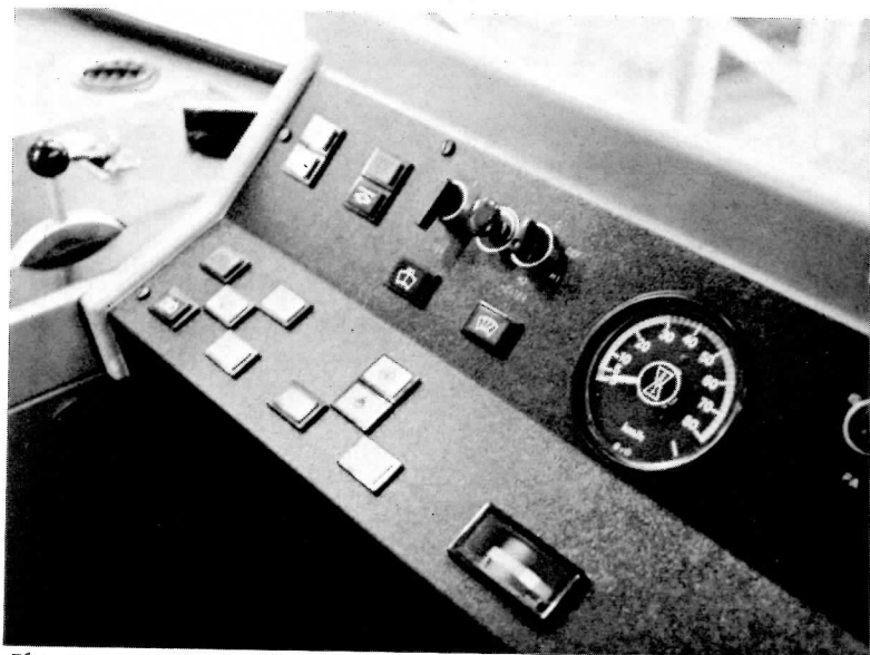
The operator's dashboard is quite straight forward, all instructions being in sign language. At the extreme left is the master controller combination brake and accelerator.
