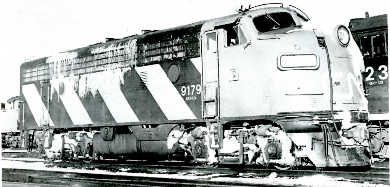
Winter visitor: CN F7Au 9179 is seen at MacMillan Yard (Toronto), Dec. 28, 1978. This unit and sister 9178, normally assigned to Western Canada, spend winters in Southwestern Ontario plow train service. Rebuilt from F7's, the modifications included upgrading from 1500 to 1750 horsepower, removal of steam generators, and wintertime application of large hoods covering the roof fans as snow protection.
